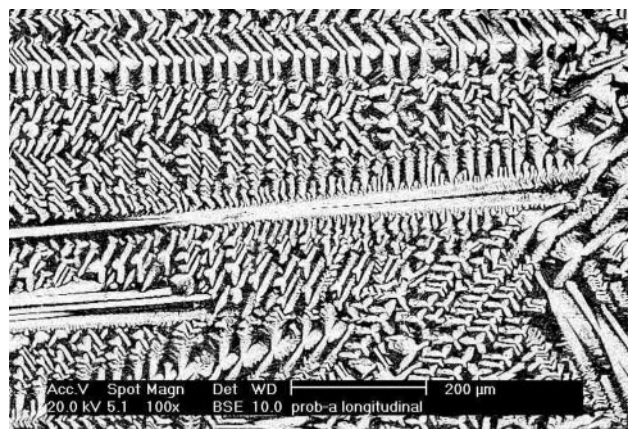
Fig. 4 Magnification of a zone of the frozen part in Fig. 2, showing the microstructure of solidifying.
